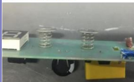
Note: The length of the live spring is 15 mm before it is assembled.
